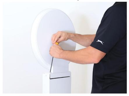
Install and tighten two bolts at the rear of the head assembly base to secure it to the pivoter.
