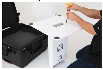
Install and tighten 4 bolts snugly (do not over tighten) using T-handle tool.
