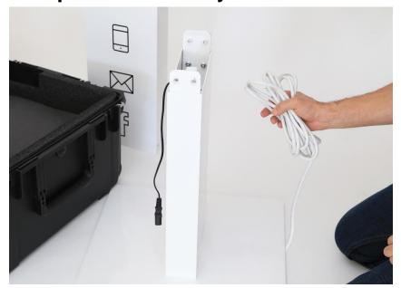
Pull the power cord from the bottom of the tube.
