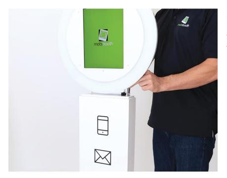
Attach the head assembly using the two front guide pins to line up the bolt holes.
