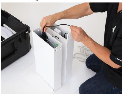
Ensure that all power cords and blocks are securely installed in the power strips within the lower tube.
